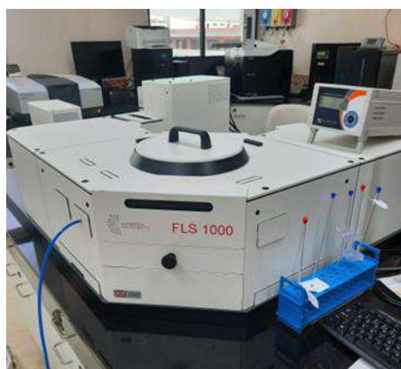
Spectrofluorometer for fluorescence and phosphorescence studies
